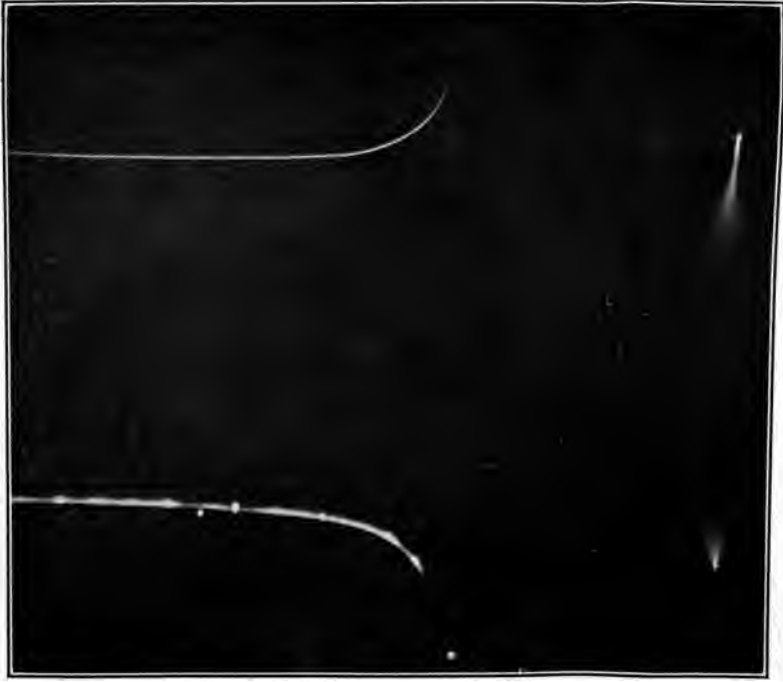
FIG. 76.—Comparison of — and + A. C. corona on wire and points. (Same as Fig. 75 with stroboscope.) (Following Fig. 74.)
